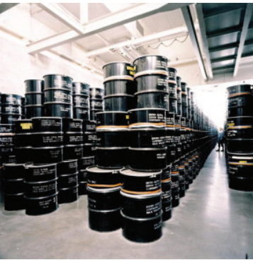
Figure 1 ILW drums (plutonium contaminated material) in storage at Sellafield
